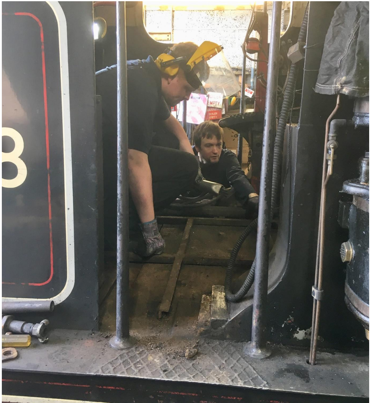
Travis (with needle gun) about to attack the cab floor. James looks on.
